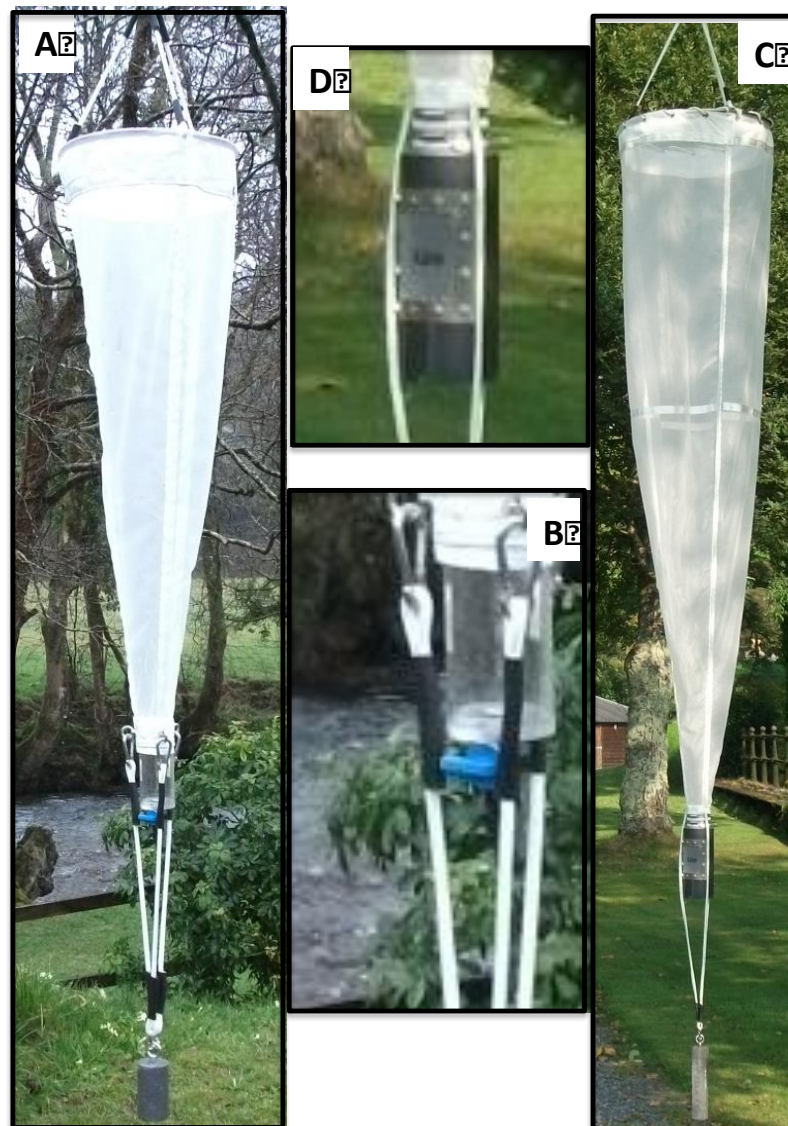
Figure 2. Plankton nets used in the DEMERSTEM Cruises. Phytoplankton net with weight attached at the bottom (A) and detail of the collector, with tap in closed position (B); Zooplankton WP2 net with weight attached at the bottom (C) and detail of the collector, with rectangular mesh window (D).
