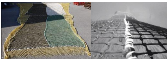
90 mm square mesh panel on the baitings of the AZUR (ashore on the left, at sea on the right) - © Ifremer
